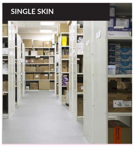
The Rackline Profile single-skin shelving consists of a panel with a double-form rear section. A closed-wall steel shelving system, the intermediate uprights are designed to support the shelves in adjoining bays.
