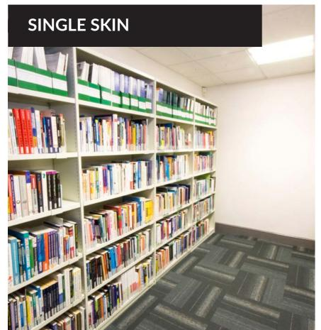
Rackline's Profile single-skin shelving is designed for efficient and secure storage in educational environments. Featuring a panel with a double-form rear section, this closed-wall steel system includes intermediate uprights to support shelves across adjoining bays.
